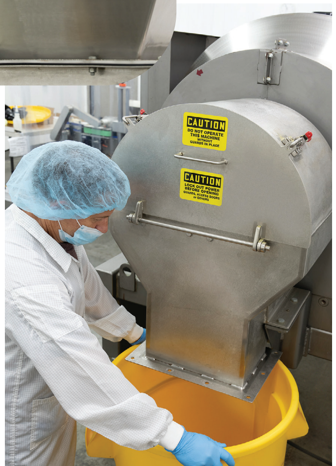
Below: The Rotary Batch Mixer loads, blends and discharges from a stationary outlet in about 15 minutes.
