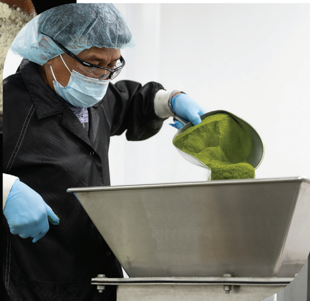
Left: Operator empties a scoop of hand-weighed powder into the mixer intake which remains stationary as the vessel turns.
